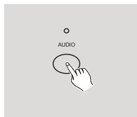
5. To return to normal mode, tap the Audio button a second time causing its LED goes out, the Audio mode is disengaged.
