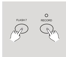
2. Tapping Flash 7 button three times while holding down Record button allows you to clear DMX channel setup and resume DMX channel to factory setting, i.e., 1-24 channel sequence.
