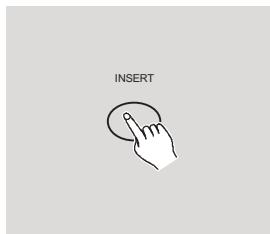
4. Tap the Insert button to insert the step you've created before, all LEDs will flash, indicating the step is inserted.
