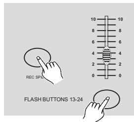
5. While pressing and holding down the Rec Speed button, tap the Flash button(13-24) that stores the program.
