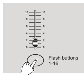
2. Tap the Flash button numbered from 1-16 to assign MIDI OUT channel 1-16, the relevant channel LED lights indicating MIDI OUT channel is set.
