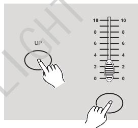
4. While holding down the Up or Down button, tap the Flash button corresponding to the DMX channel of the scene you wish to modify until you reach the desired intensity value read from the Segment Display. Then you may tap the Flash buttons until you are satisfied with the new scene.
