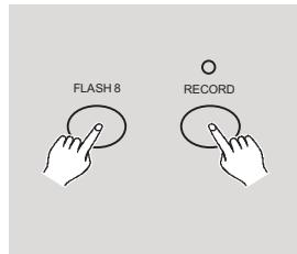
2. Tapping Flash 8 button three times while holding down Record button allows you to access DMX channel setup. The Segment Display reads the current DMX channel.
