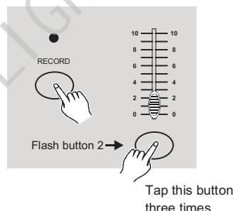
1. Tap the Flash button 2 three times while holding down the Record button, the Segment Display reads "CHO" indicating MIDI OUT channel setup is available.
