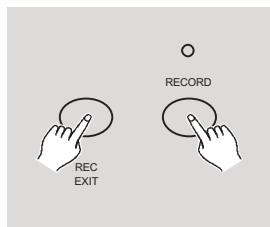
8. You can continue programming or exit. To exit Program mode, tap the Exit button while holding down the Record button, the Record LED should go out.
