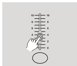
5. Move the Channel slider to adjust the output of the current program.
