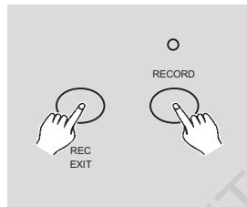
Press and hold down the Record button. While holding down the Record button tap the Rec Exit button to exit MIDI setting.
