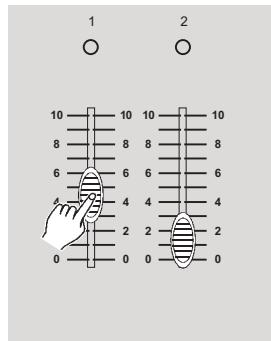
3. Create a desired scene using Channel Sliders 1-24. At 0% or DMX 0, these sliders should be at 0 position, and at 100% or DMX 255, these sliders should be at 10 position.
